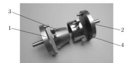
Fig. 1. Components of the investigated sleeve-shaft neck friction joint: 1 – lower pressure plate grip of the model, 2 – upper grip of the model, 3 – shaft neck, 4 – sleeve
